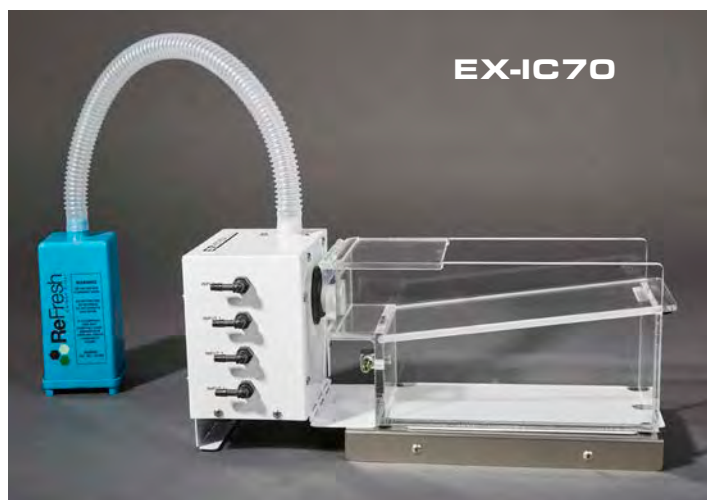
Optional EX-IC70 Exhaust Cube features an internal blower that captures waste gas from our vented chamber and up to four breathing devices.
